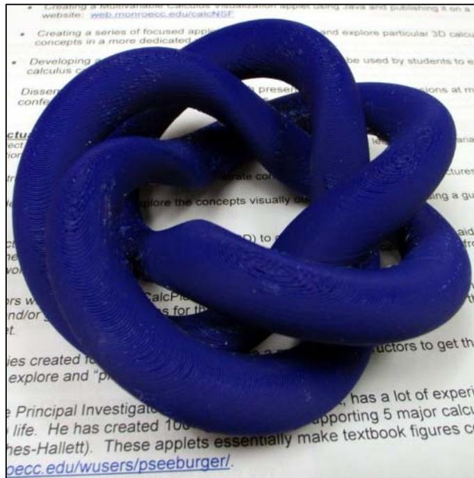
In order for the STL file to work well with the 3D printer, the surface must be given sufficient thickness. To address this issue, CalcPlot3D will automatically give the thickness you specify to a surface before creating the STL file. The applet essentially creates a closed solid to represent the surface.
